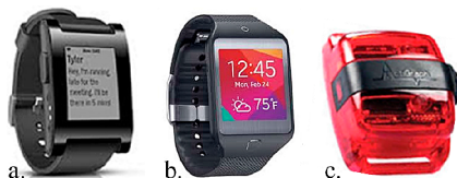
Figure 1. (a) Pebble Classic, (b) Samsung Gear and (c) Actigraph WGT3X-BT devices
