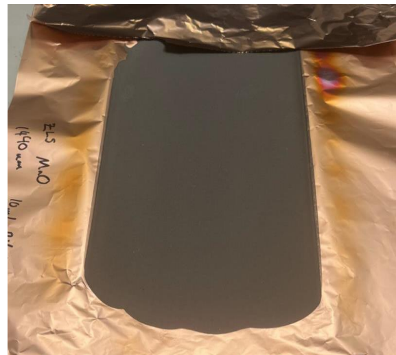
Zelos Cathode coating on low-cost foil
