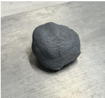
Typical Zn Viscosity is not suitable for standard roll-to-roll equipment
