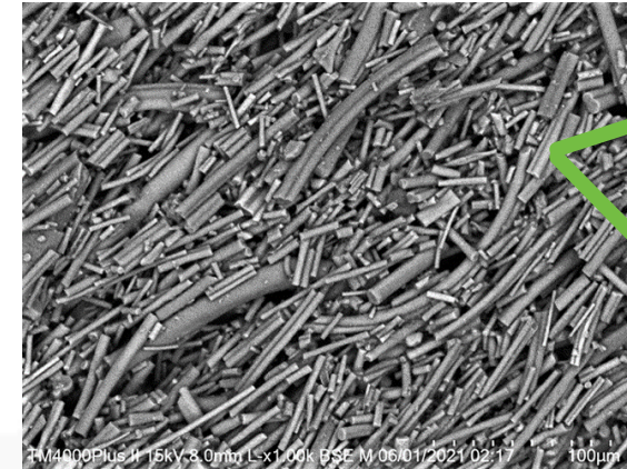
Novel Sponge Like Si Structure Fiber ~3µm Diameter
