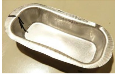
First metal sheet forming tests (aluminium & steel)
