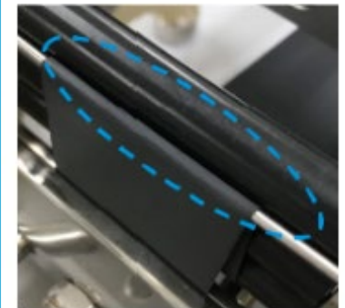
NEOFLON VT-475 with homo PVdF Wounded w/o cracking
