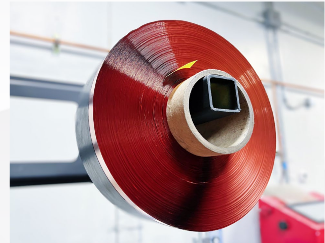
200 m Roll of Graphite Anode
