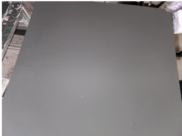
30cmx30cm cathode Composition: 96% NMC622, 2wt% carbon, 2wt% PVDF
