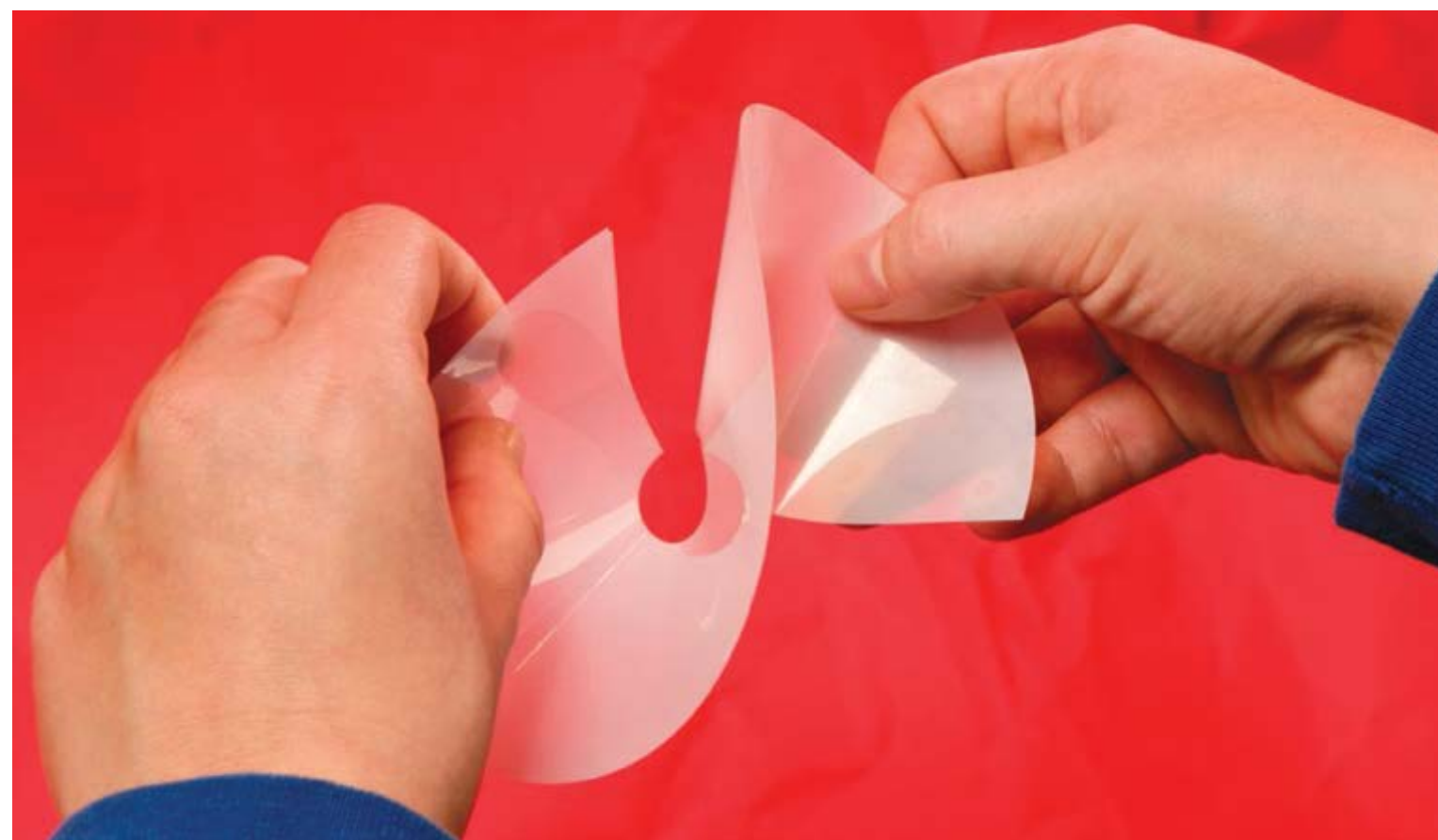
ENrG Ultra-Thin, Flexible Ceramic Substrate: 40μm
