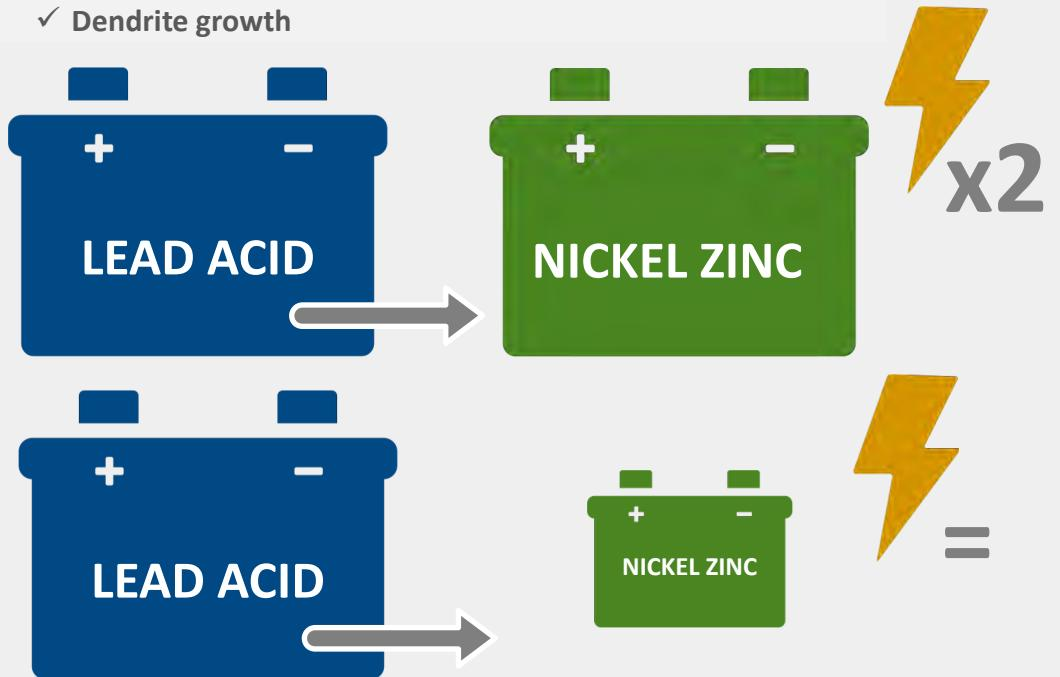
A Nickel Zinc (NiZn) battery can give 2x capacity and cycle life in the same size or the same capacity and 2x the cycle life as a Lead Acid battery in half the footprint.
