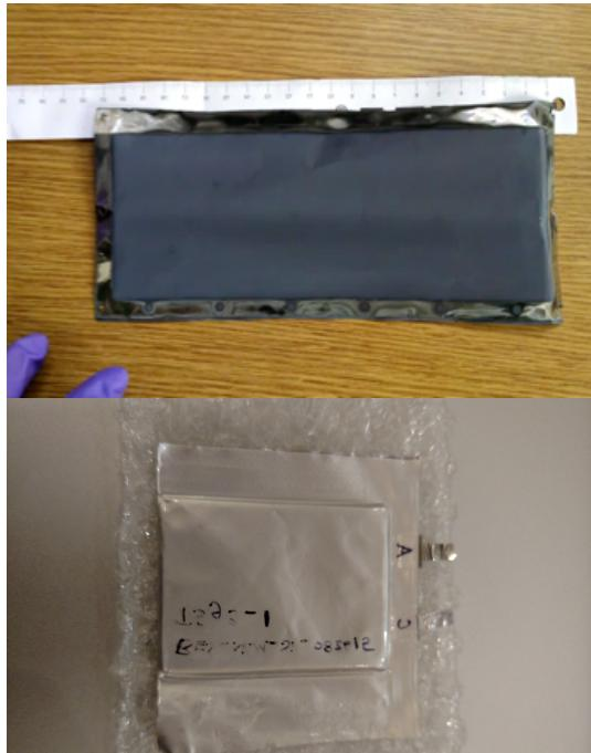
Single step CVD manufacturing, deposition directly on current collector
