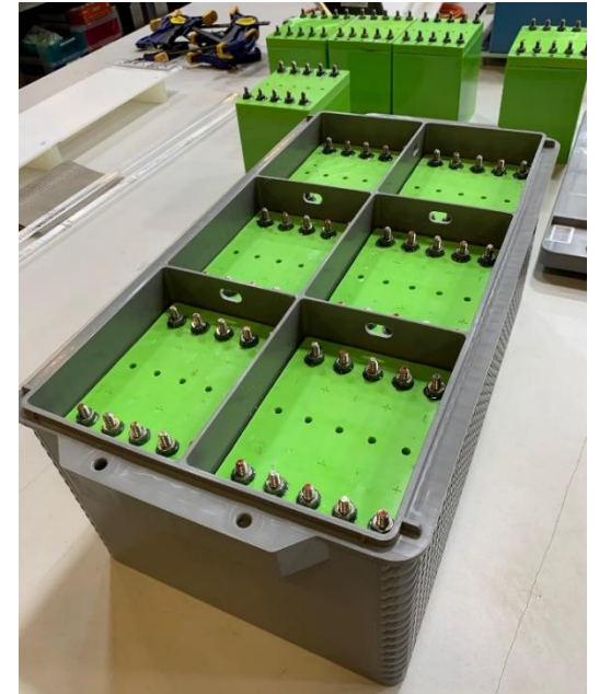
Populated 48V 8D (fore) and sealed (activation ready) 8.5V subcell (rear)
