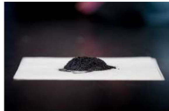
Recycled cathode powder ready to be used in a new battery. Courtesy of University of California San Diego
