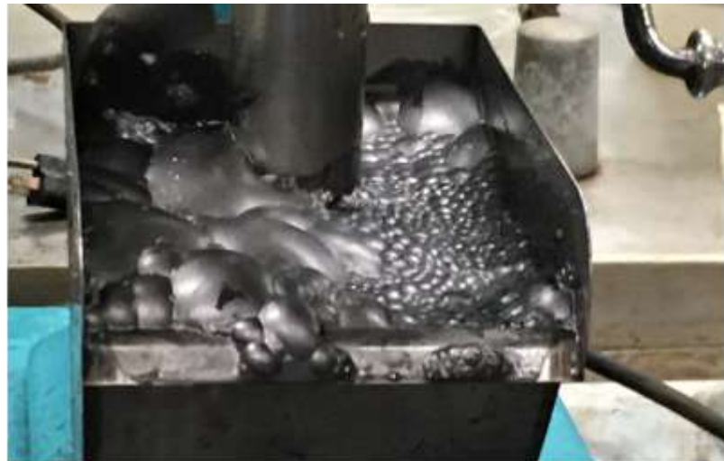
A laboratory scale froth flotation unit is used to separate anode powders from cathode powders. This is the first step in recovering the anode powder. Courtesy of Argonne
