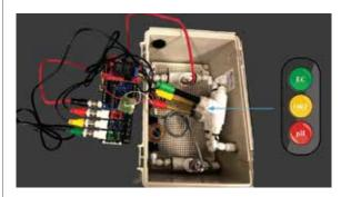
Figure 1. Water quality sensor node. Drinking water enters on the bottom right and travels through the plumbing. Plumbing includes a pressure sensor, temperature sensor, and pH, ORP, and EC probes. Water exits using the top right outlet. The 'electrical stack' pictured typically sits in the box, but is removed so the plumbing is more easily visualized.
