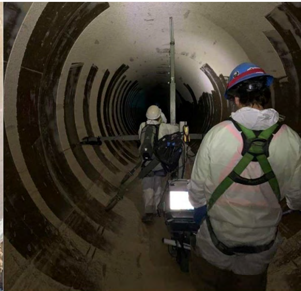
Figure 7. PICA operator monitoring the EM data as it's collected during the August 2022 NFT inspection of GLWA's 120-inch PCCP Transmission Main.
