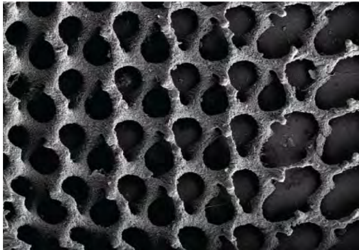
A close up of 3D printed synthetic bone mimicking trabeculae, a major part of natural bone. Credit: Roohani et al. , Advanced Materials (CC BY-NC 4.0)
