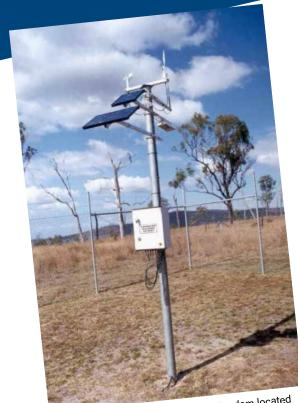
A PDS Automatic Weather Station at a dam located near Brisbane, Australia. Automatic Weather Station consists of a DT50 data logger, solar panels, radio modem and meteorological sensors. Source: Pacific Data Systems Pty Ltd, <u>http://www.pacdatasys.com.au</u>. *Credit: Wikimedia Commons.*
