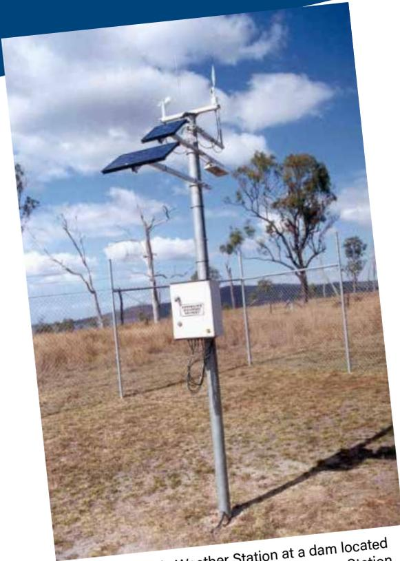
A PDS Automatic Weather Station at a dam located near Brisbane, Australia. Automatic Weather Station consists of a DT50 data logger, solar panels, radio modem and meteorological sensors. Source: Pacific Data Systems Pty Ltd, <http://www.pacdatasys.com.au>. Credit: Wikimedia Commons.
