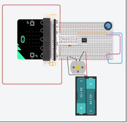
Go to <a href="https://makecode.microbit.org/#editor">https://makecode.microbit.org/#editor</a> and create the program (shown below). This program will measure the potentiometer position and adjust motor speed accordingly.
