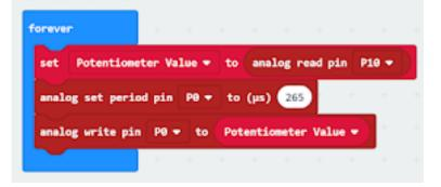
Send the program to the Micro:bit. Connect the Micro:bit to the computer and hit save on the file name. This will download the file (as well as save it for later). The downloaded file can be transferred to the Micro:bit by drag and drop (the Micro:bit behaves like a flashdrive).
