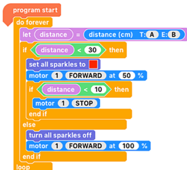
Figure 2. Example of a working code and explanation of the code for the collision avoidance design challenge.
