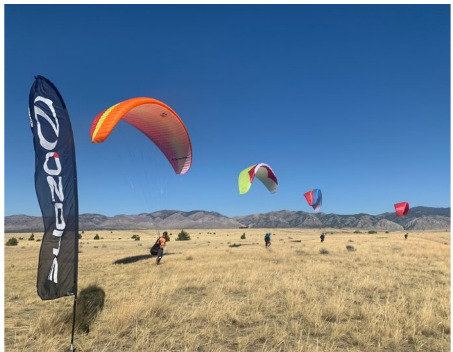
Figure 3. Aircraft with non-rigid wings (note the ram air opening on the leading edge). A group of paraglider pilots “kite” their wings in a steady breeze.
