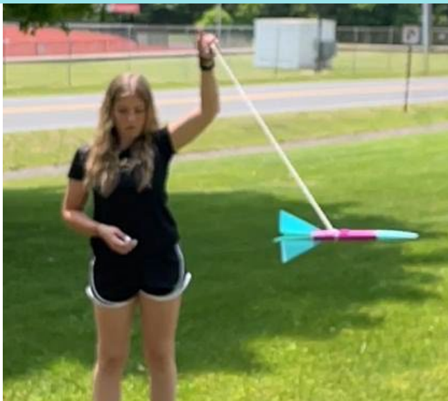
Figure 8. A student tests the stability of their class rocket. They swing it around by its center of gravity, observing if it orients itself correctly—this one passes the test!
