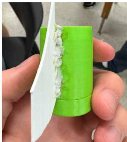
Figure 4. A small section of a rocket fuselage with the fin and engine cap attached. You can also see that students were experimenting with welding the fin to the fuselage.
