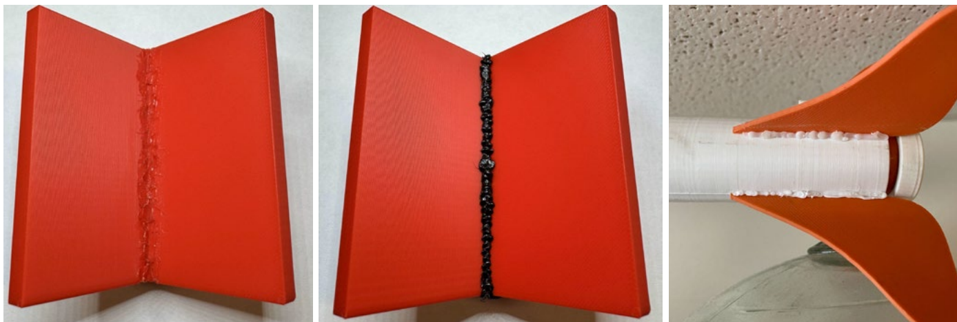
Figure 7. Examples of welding and “brazing” 3D-printed components (left and center, respectively) and a combination of both techniques on the final rocket assembly (right).
