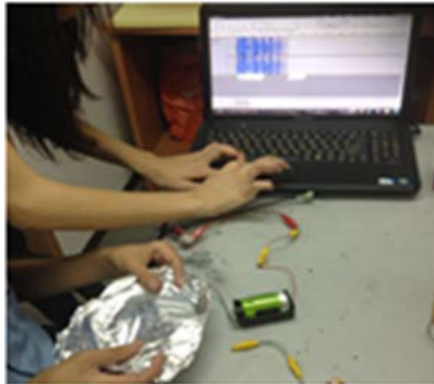
Testing a magnetic microphone using the Audacity software
