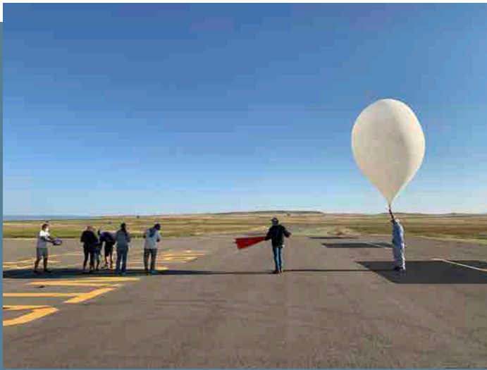
A latex pressure balloon about to launch. Pressure balloons have a sealed bottom and pop at max altitude.
