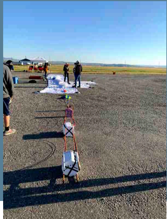
Payload string and balloon ready for flight. Several tarps and sheets are placed down first to protect the balloon. Socks filled with sand hold the sheets and tarps down.
