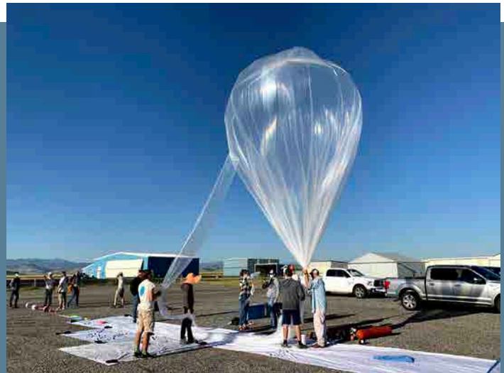
A zero-pressure balloon about to launch. A zero-pressure balloon has an opening at the bottom and will not pop. Zero pressure balloons rise until they reach neutral buoyancy then float. They must be flipped upside down to descend.
