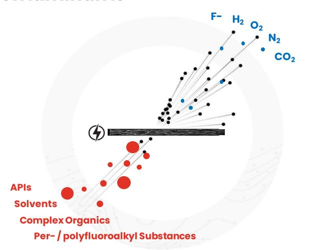
Electricity is applied to advanced catalysts to trigger **direct and indirect oxidation**.
