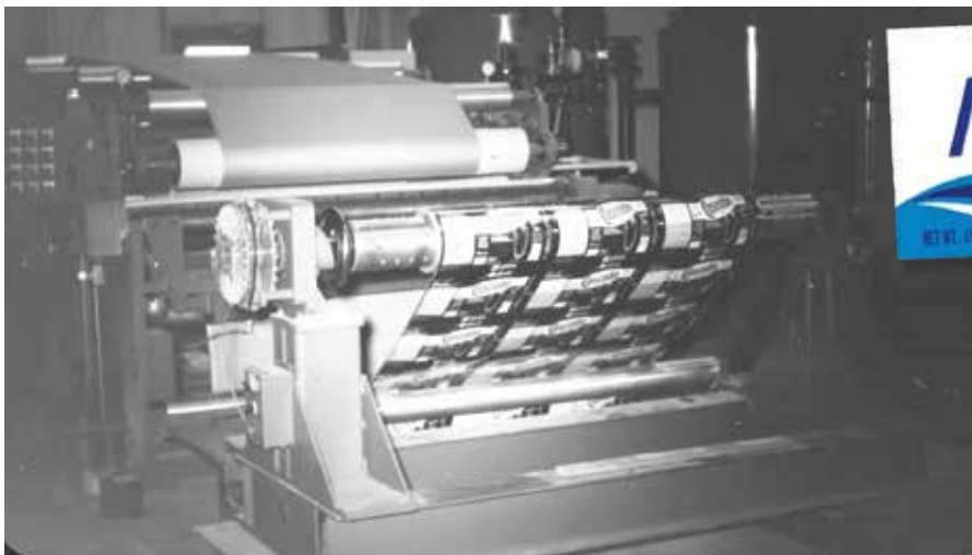
American Packaging Corporation's slitter machine cutting Cascade® detergent rollstock
