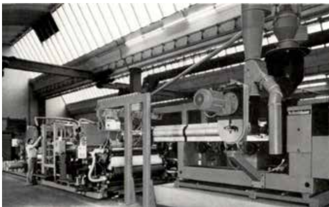
New automatic controlled chill roll film line from Reifenhäuser
