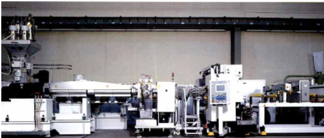
Thermoforming sheet line for processing of PLA-based bio raw materials in 2007. Photo courtesy of Reifenhäuser.
