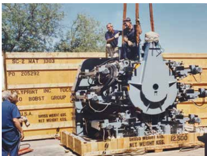
Poly Print, Inc.'s first press installation, the CI section of a Schiavi Padini wide web printing press in 1992. Photo courtesy of Poly Print, Inc.
