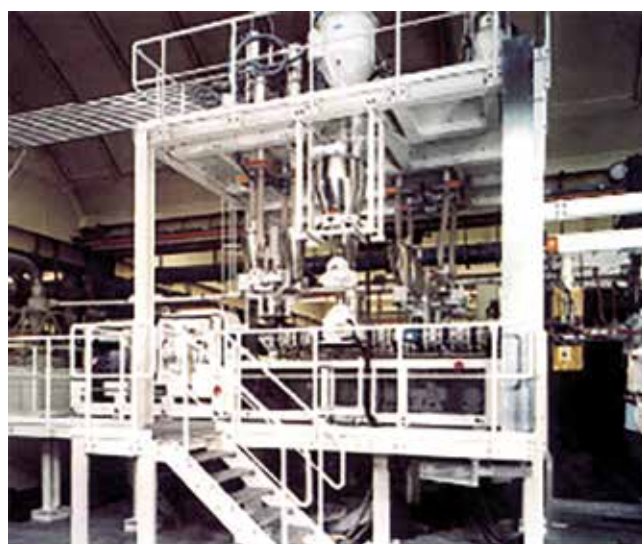
Reifenhäuser's REIfill direct extrusion line with “Reitrunder” twin-screw extruder to produce filled multilayer sheet, thermoforming sheet, and cast film
