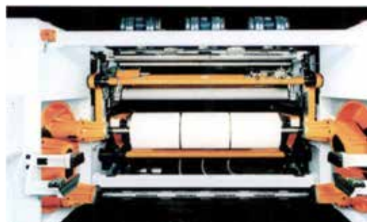
High performance MIDES series rotary arm winder from Reifenhäuser
