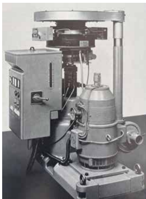
Reifenhäuser vertical extruder “SV 050.1” for film lines
