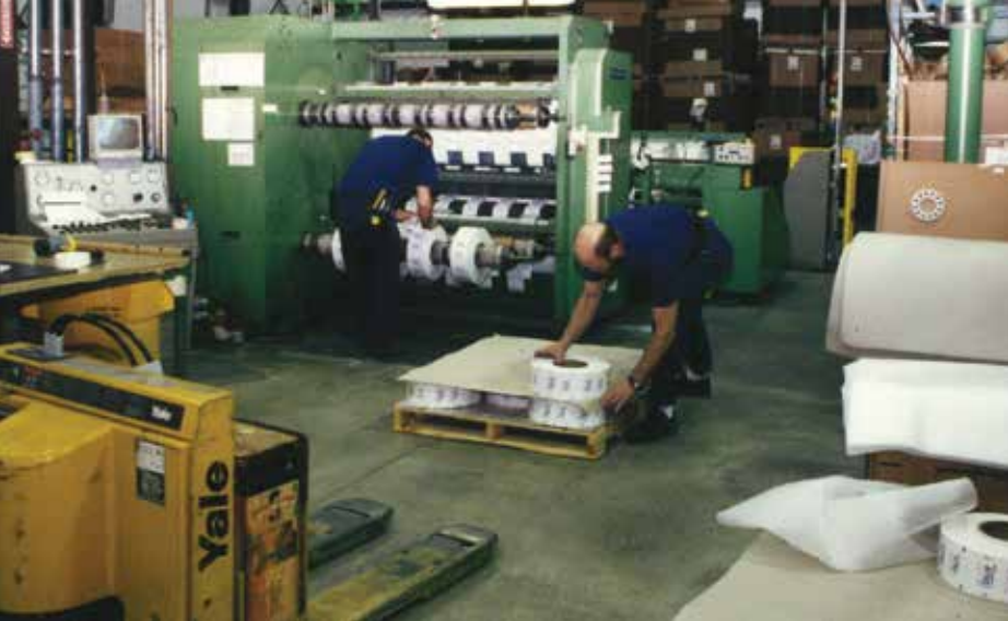
American Packaging Corporation's slitter machine cutting Ivory soap wrap
