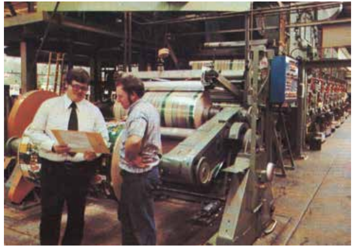
American Packaging Corporation rotogravure press printing Cascade® detergent in 1980
