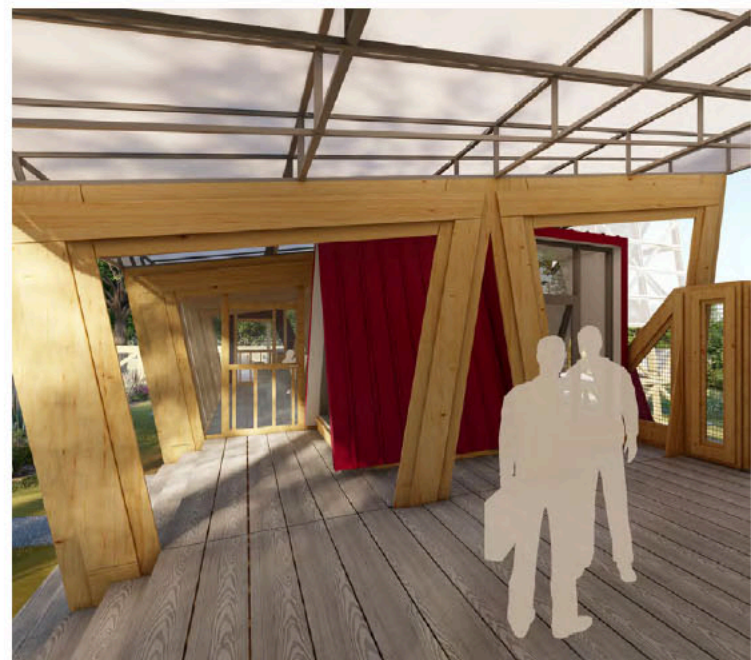
Community Hall: Prefabrication for Transport and Adaptive Reuse Three sets of trusses are transported, stacked, and clipped together.
