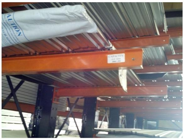
Note arm Load Capacity Rating & train forklift operators
