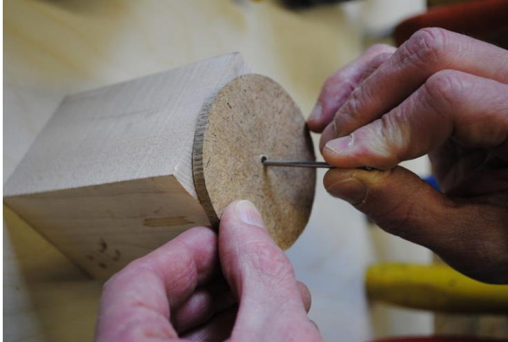
Figure 15 - A homemade round template set against the end of a blank with a nail inserted through its middle hole.
