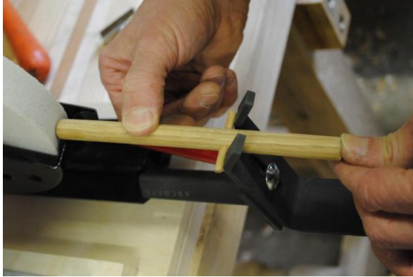
Figure 6 - A man demonstrating how to use a homemade dowel jig to set the distance between the base of the Vari-grind jig and the grinding wheel. Instructions follow.
