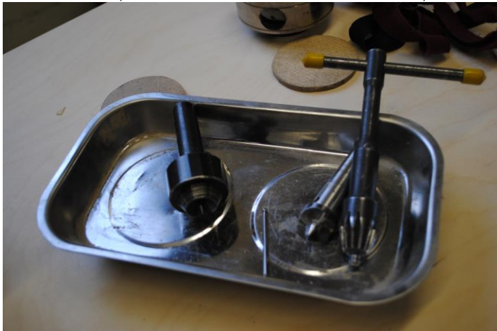
Figure 14 - A close-up of the small-parts tray at the workstation. This one holds a nail, a live center used in the tailstock, a drive center used in the headstock, and a chuck wrench.
