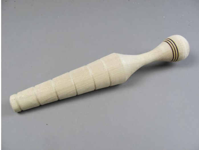
Figure 21 - A garden dibble to measure the depth of dirt for planting bulbs. V-cuts are at 1/2", 1-1/2", 2-1/2", 3-1/2", 4-1/2", and 5-1/2". The top end is a handle, contoured for comfort.
