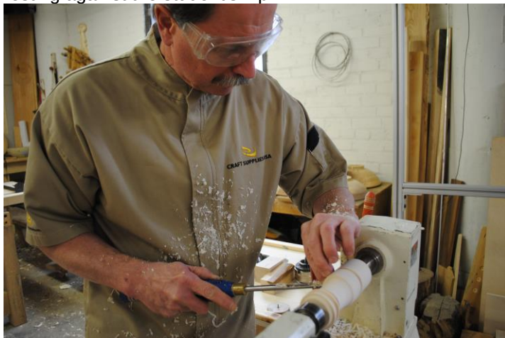
Figure 20 - A blind student is at the lathe, holding a spindle gouge, ready for a cut. His left hand is on the wood and the gouge flute. His right hand is holding the spindle gouge, the handle of which is resting against the student's hip.
