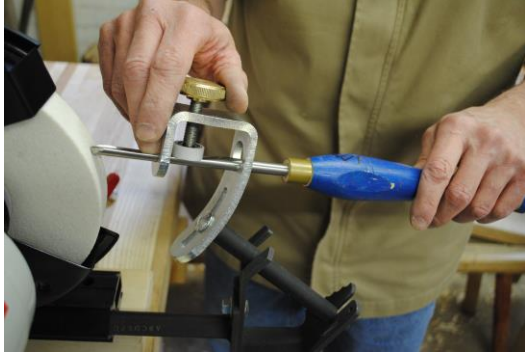
Figure 4 - A man demonstrating the Vari-grind jig by holding a spindle gouge against the grinding wheel.
