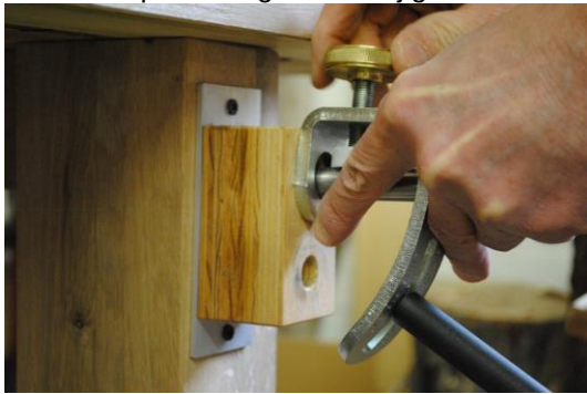
Figure 5 - A man demonstrating how to use the wooden block to determine the correct length that the tool should be protruding from the jig. Instructions follow.
