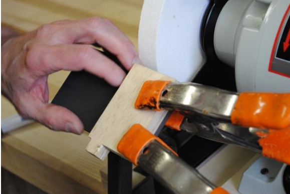
Figure 9 - A jig mounted to the platform, being held by two pressure clamps.
