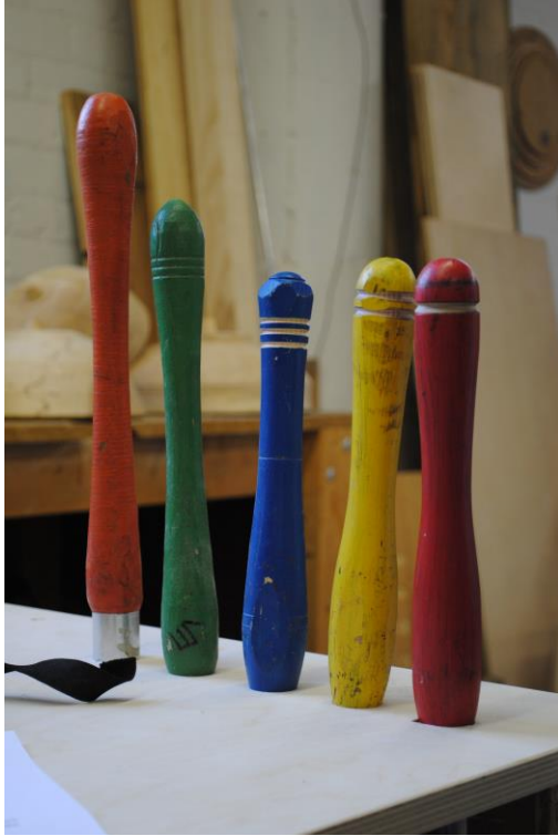
Figure 13 - Five turning tools, showing coves cut at the end of each tool to identify it, in order of use.
