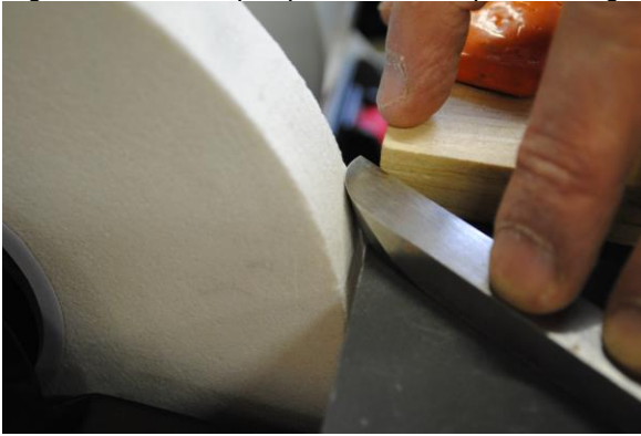
Figure 10 - A scraper placed on the platform against the jig.
