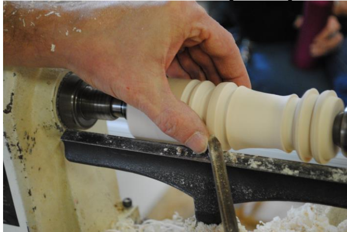
Figure 19 - This image shows the hand placement on the wood spinning on the lathe, with the thumb anchored on the toolrest and the fingers wrapped around the wood cylinder. The thumb feels the recess of the cove, and the flute of the turning tool is against the thumb to follow along while making the next cut.
