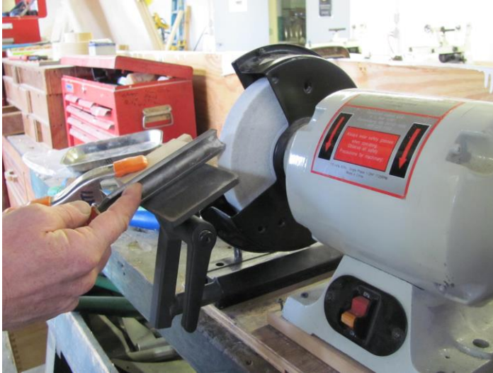
Figure 11 - A man holding a roughing gouge on the platform of the sharpening grinder. The flute faces 3 o'clock in the center of the platform and up against the jig.
