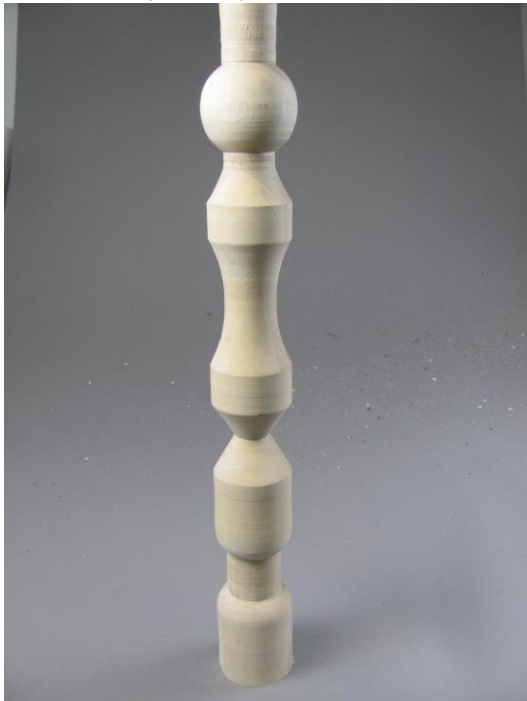
Figure 18 - The image represents a demonstration stick, a useful tool for helping the any turner understand the types of cuts and shapes. It is an oversized large spindle with straight cuts, beads, coves, flat surfaces, V-cuts, and rounded corners.
