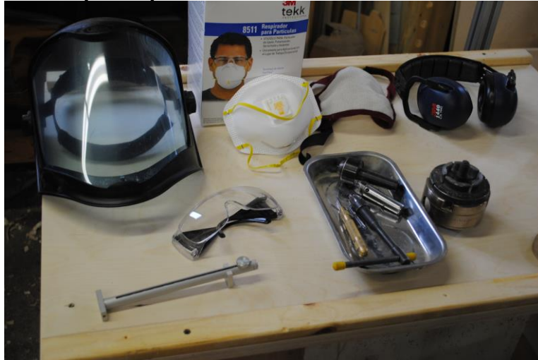
Figure 12 - Tools and equipment laid out on the top of a workstation. Included are a face shield, mask for dust protection, earphones to minimize noise, a depth gauge, a chuck, and various small tools in a shallow tray so they won't roll around.
