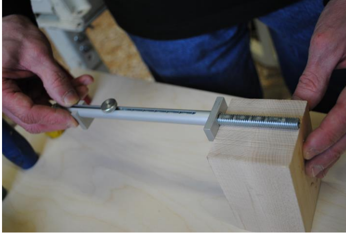
Figure 17 - A click stick resting alongside the end of a wood blank. The end of the click stick is flush with the opposite edge of the blank, and its metal stop has been moved up flush with the near edge of the blank.
