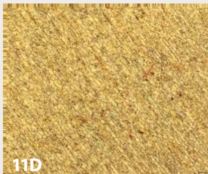
Magnification 100X, wood surfaces cut with CPM 15V gouge.
