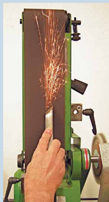
On the Big Tree Tools flat-platen belt machine, both sides of a skew chisel can be ground and sharpened from a single jig position. The belt machine works equally well if the edge of the skew is straight or curved.
