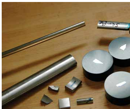
Sections of lathe tools embedded in composite materials and prepared for emission (spark) test.
