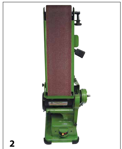
For this modification, unpack the parts but do not mount the disk sander or its table. Also, remove the back cover and bottom dust port, the sanding-belt guard, and the drive-belt cover.
