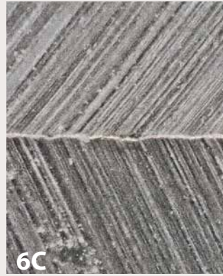
6C Edge view of skew chisel edge, ground (200X).
