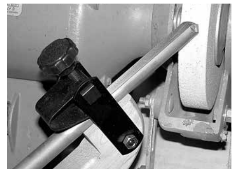
A jig may be helpful in some situations of learning to grind.
