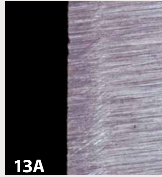
Cutting edge of a M2 HSS skew, ground and honed (200X).
