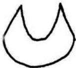
15. Thin skew-like edge can cause vibration 16. Additional mass behind edge reduces vibration
