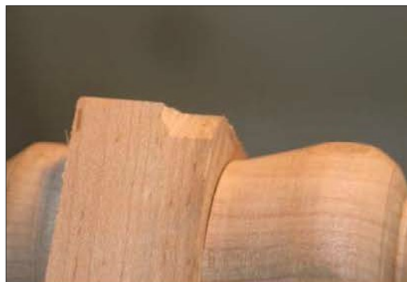
Roughing the face grain blank
