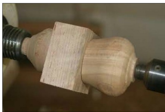
Blank on Morse taper Mandrel
