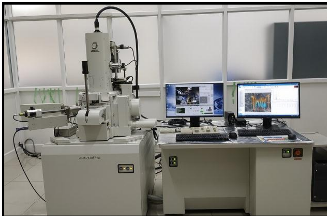
Figure 3: Representative image of the front-view image of a JEOL JSM-7610FPLUS scanning electron microscope (SEM) equipped with an Energy Dispersive Spectroscopy (EDS) detector. The cylindrical EDS detector, positioned above the specimen chamber, facilitates elemental analysis of microscopic samples
