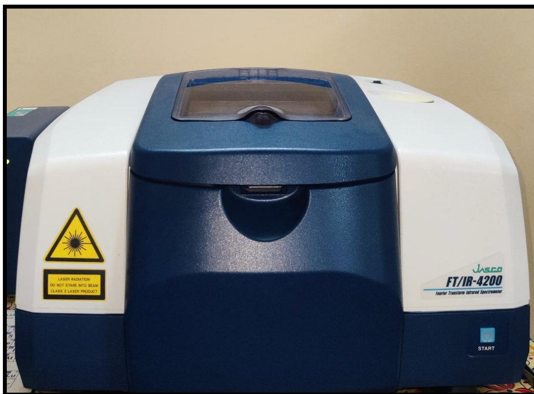
Figure 4: The representative figure depicts a Jasco FTIR 4200 spectrometer employed in this study for the identification of functional groups in biological samples. The spectrometer operates by directing infrared radiation through the sample, causing specific absorption based on its molecular composition. The resulting spectrum, generated by interferometer modulation and detected by a sensitive detector, provides a unique fingerprint for the identification and quantification of targeted functional groups.
