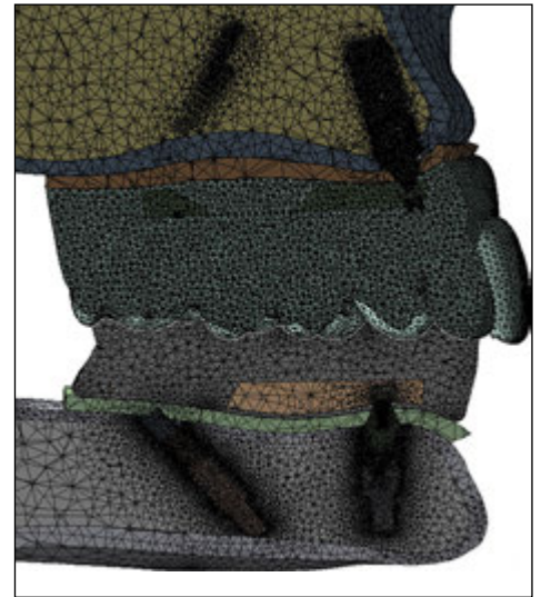
FIGURES 2. A cross section from the model to which the mesh process is applied.
