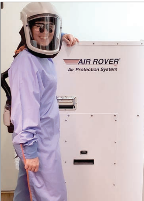
Dr. Kaban utilizes a heavy-duty, hospital-grade air scrubber (Air Rover APS2000) that purifies the air in her office at a rate of 10,000 cubic feet of air in 23 minutes or 2,000 cubic feet per minute. The air is purified through HEPA filters and UV-C lights.
