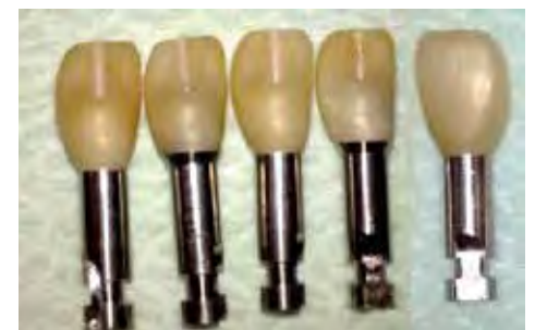
Lateral incisor study models on replicas: partially stabilized zirconia (PSZ) direct, PSZ on titanium (Ti) base, fully stabilized zirconia (FSZ) direct, FSZ on Ti base, Procera.
