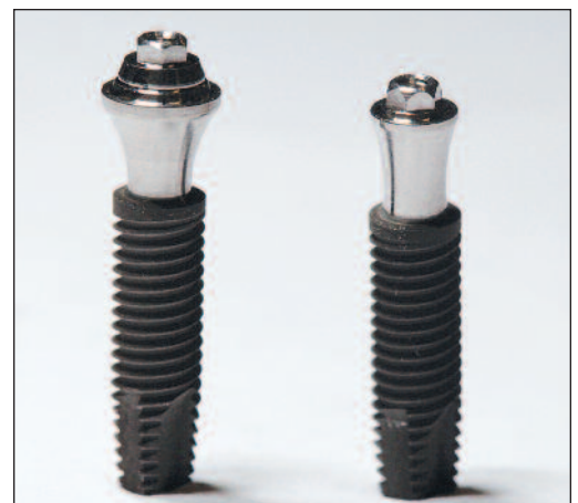
Figure 1: Prosthetic abutments tested in the study (left, standard diameter; and right, small diameter).
